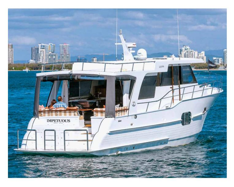
Approaching the 530 from astern, I caught a glimpse of the single-level cockpit and galley-cum-saloon to the semi-fly helm and through the wide windscreen. And instantly I saw the appeal – the layout offers the driver a raised helm position with more headroom under the decks without losing the social flow to the entertainment zone
