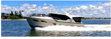
Volvo D11 670 HP. Topspeed 22 knots Semi-displacement hull
